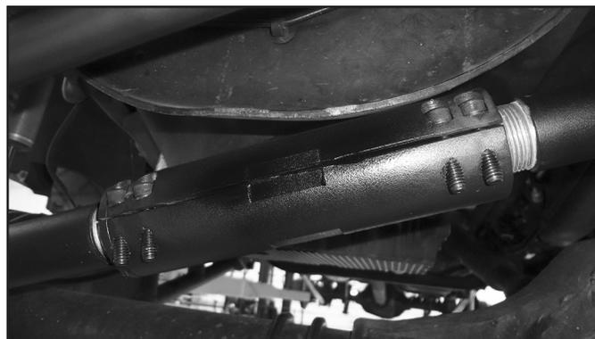
23. Attach the axle mount to the track bar. It may be necessary to have an assistant turn the wheel to get the mount to line up. Square the mount up to the factory joint. Attach with factory nut. Tighten to 184 ft-lbs
