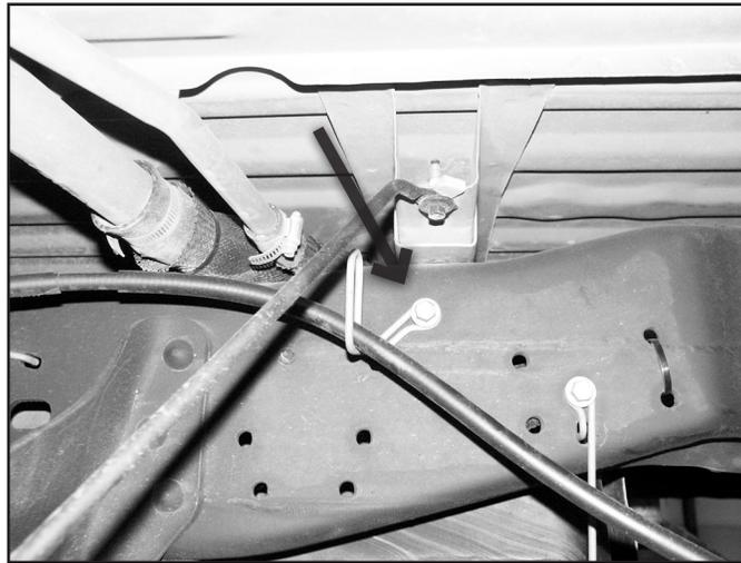
45. The brake lines may require additional slack. Located the factory bracket on the axle. Using an adjustable wrench, carefully bend the bracket so the fittings are positioned vertical to allow more slack. (Fig 14)
