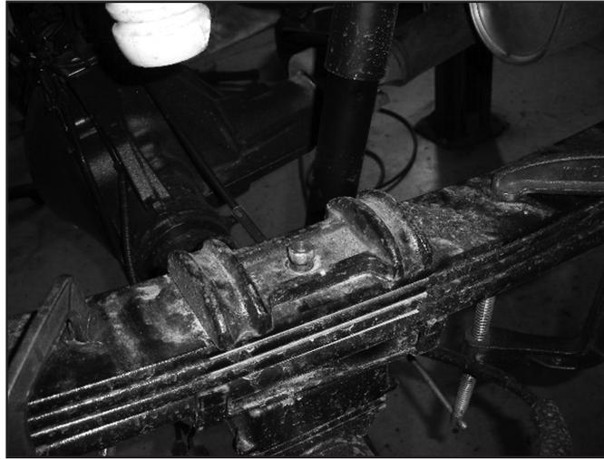
40. Remove the factory lift block. It will not be reused.
