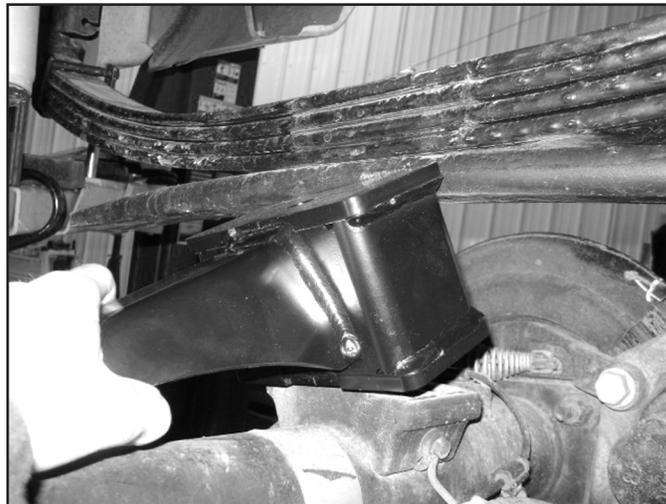
43. Repeat block installation of the driver's side. Take care not to over extend the brake lines.
