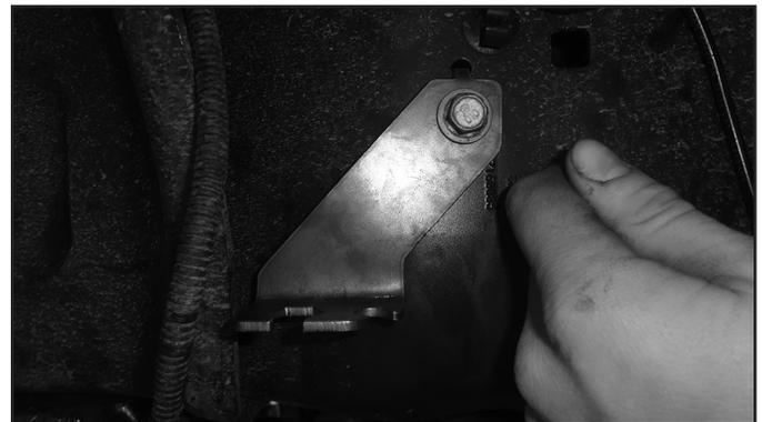
40. Remove the clip holding the brake line to the factory bracket. Save the clip for later installation.
