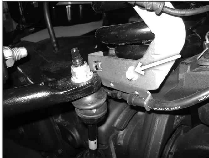
7. Remove the bolts attaching the front brake lines brackets to the frame and save the hardware (Fig. 2). Attempt to not bend the brake lines as much as possible. Remove the ABS line from the brake line bracket.
