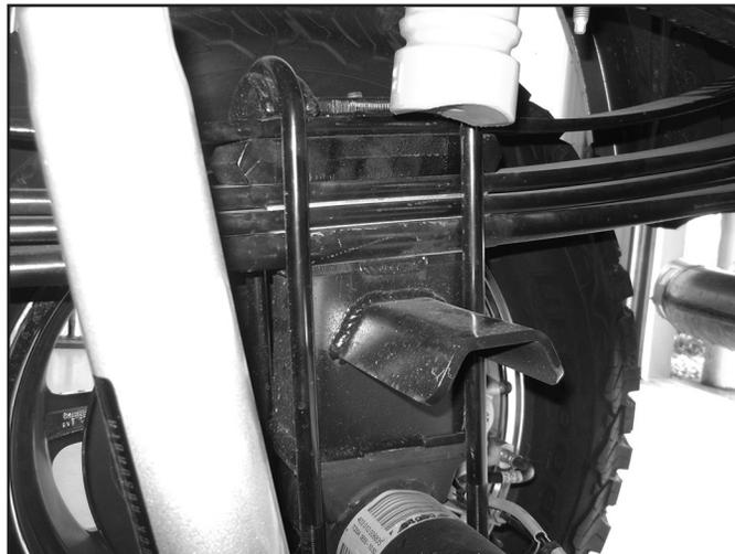
104. Raise the axle to engage the block spring alignment pins. Fasten the entire assembly with the provided u-bolts, washers, and nuts. Snug but do not torque the u-bolts at this time. (Fig 29)
