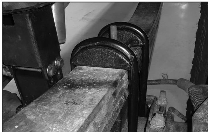
119. Install the new spring in the vehicle with the OE bolts. Use the provided 7/8" SAE Washers as spacers as needed for the front leaf spring bushing (use one on each side of the leaf spring bushing). Leave hardware loose. All of the spring pivot bolts will be torqued with the weight of the vehicle on the springs.
