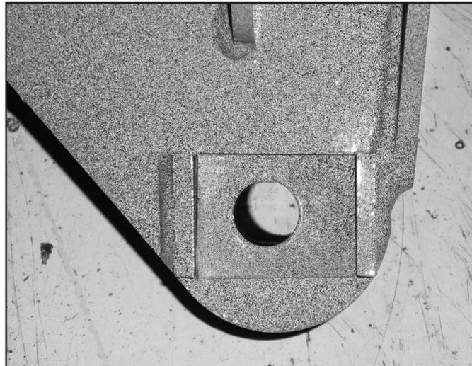
54. Install the transfer case skid plate drop bracket on the driver side using the factory hardware into the J-nut in the frame. The bracket should be slanted towards the rear of the vehicle. Attach the transfer case skid plate to the J-nuts in the frame on the passenger side using the factory hardware. Attach the transfer case skid plate to the drop bracket on the driver's side using the 3/8" hardware from Bolt Pack 987 in the Indexing Ring kit. Torque to 20 ft-lbs (Figure 16).
