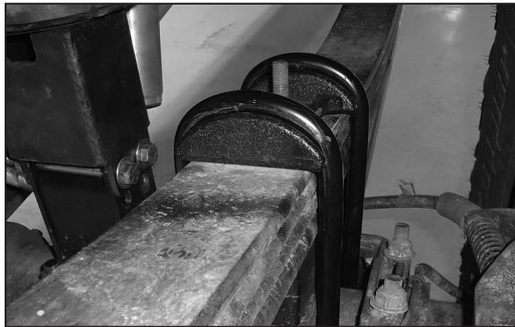
88. Install the new spring in the vehicle with the OE bolts. Use the provided 7/8" SAE Washers as spacers for the front leaf spring bushing (use one on each side of the leaf spring bushing. Leave hardware loose. All of the spring pivot bolts will be torqued with the weight of the vehicle on the springs.
