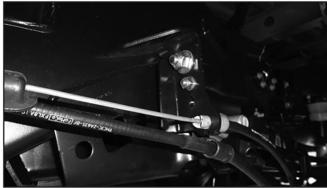
123. Install the passenger side E-brake cable into the bracket, make sure the tabs on the cable lock the cable into place.
