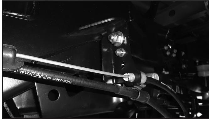
92. Install the passenger side E-brake cable into the bracket, make sure the tabs on the cable lock the cable into place. (Figure 25)
