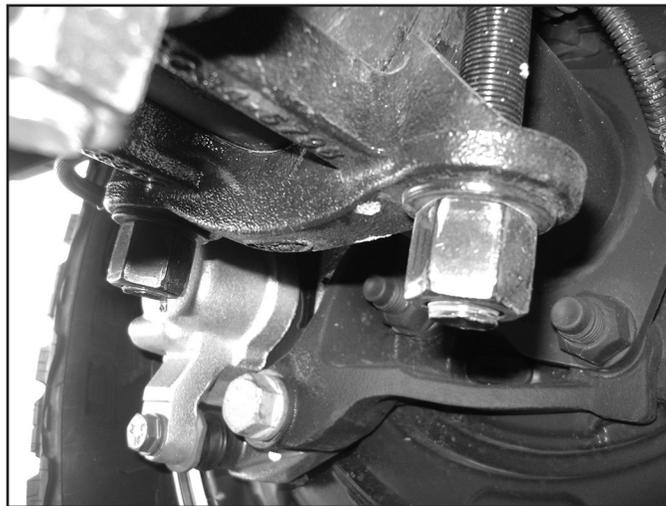
81. Repeat block installation of the driver's side. Take care not to over extend the brake lines.
