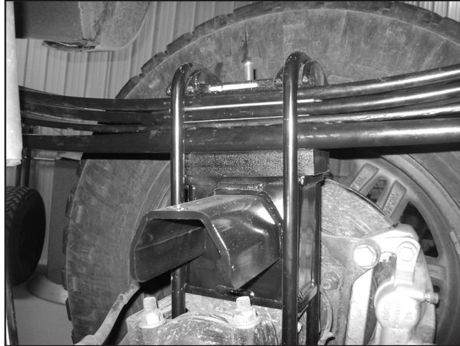
80. Raise the axle to engage the block spring alignment pins. Fasten the entire assembly with the provided u-bolts, washers, and nuts. Snug but do not torque the u-bolts at this time.
