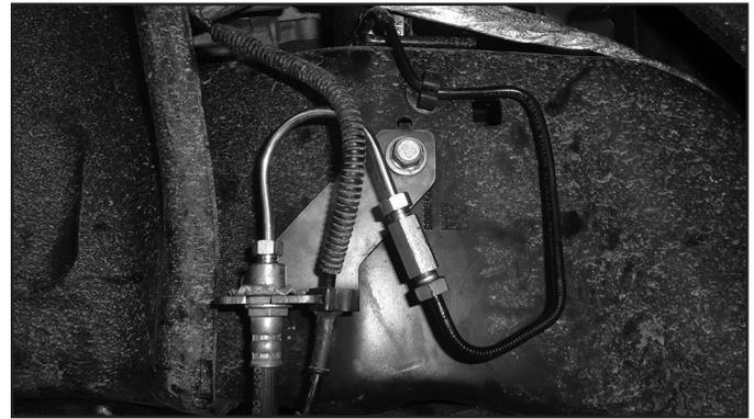
46. Attach the ABS wire to the new brake line bracket. The rubber grommet may need to be slid up the ABS line, use silicone spray to help aid in moving the rubber grommet. (Fig.12)
